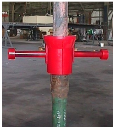
Place pin end inside guide and make up the joint.
